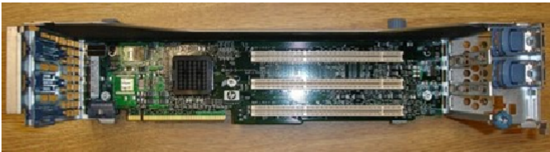
Example of a HP ProLiant PCI riser cage, removed from server chassis
