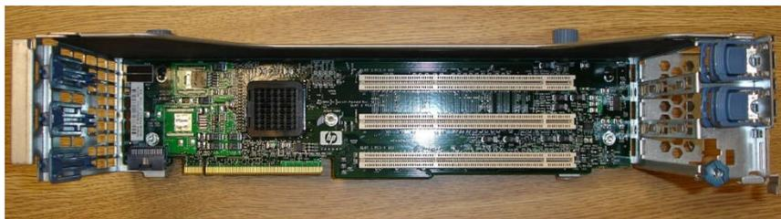
**Example of a HP ProLiant PCI riser cage, removed from server chassis**
